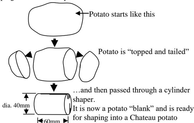
**Figure 3.** Pre-shaping the potato ready for processing by the Chateau potato shaping machine 3
