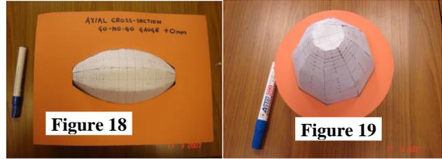
Using go-no-go gauges to check accuracy of the Chateau potato cardboard models in two perpendicular axes
