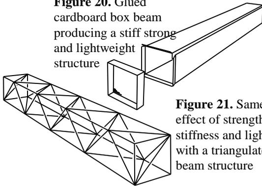
**Figure 21.** Same effect of strength, stiffness and lightness with a triangulated box beam structure
