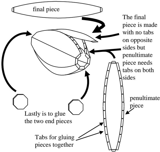
**Figure 15.** Construction of the cardboard potato
