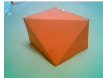
**Figure 10** After making engineering drawings and working out true lines and true planes the students construct a cardboard model of the cut box
