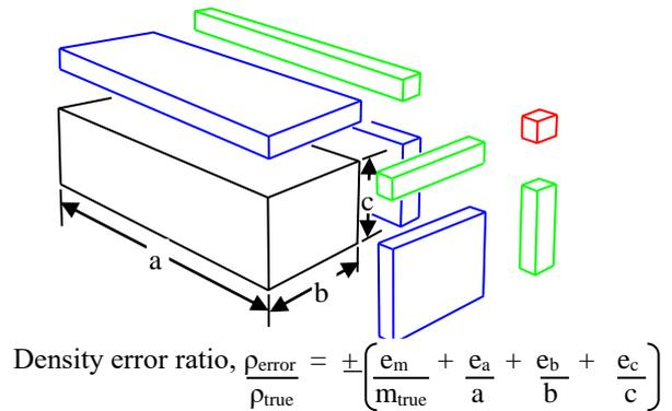
**Figure 6.** Measuring the density of potato substance and the errors of its measurement.
