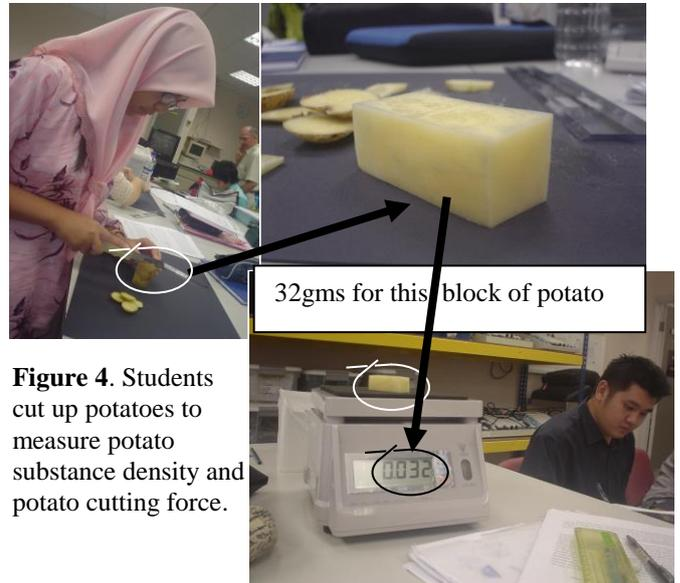
**Figure 4.** Students cut up potatoes to measure potato substance density and potato cutting force.
