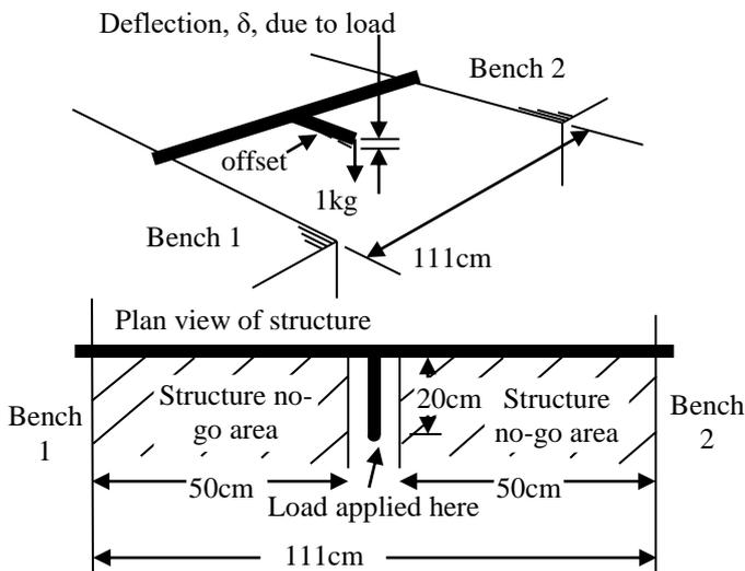
**Figure 23.** Specification of bridge structure to be built by students working in groups not exceeding 3 students
