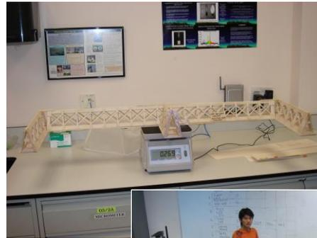
**Figure 24** Bridge structure under test for its mass measurement
