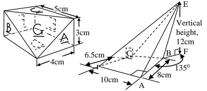
**Figure 9.** True line and true plane problems using a cut box and a pyramid
