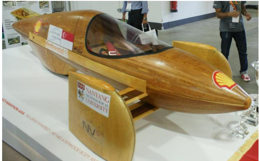
In fact since wood has a lower density than steel and aluminium it has a higher stiffness and strength per kilogram when compared to steel and aluminium when used in bending since the 2nd moment of area is higher per unit weight. Wood is also a wonderful prototyping material. You can cut it, saw it, laser it, shape it, drill it, glue it, bend it, laminate it, screw it, nail it, join it and smooth it. You can change your mind and cut it apart and modify it and reglue it.
